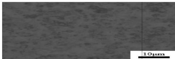
图1 2Cr13钢带冷轧状态下的金相组织 Fig.1 Microstructure of 2Cr13 steel strip after cold rolling
