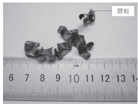
(c) 挤裂切屑
